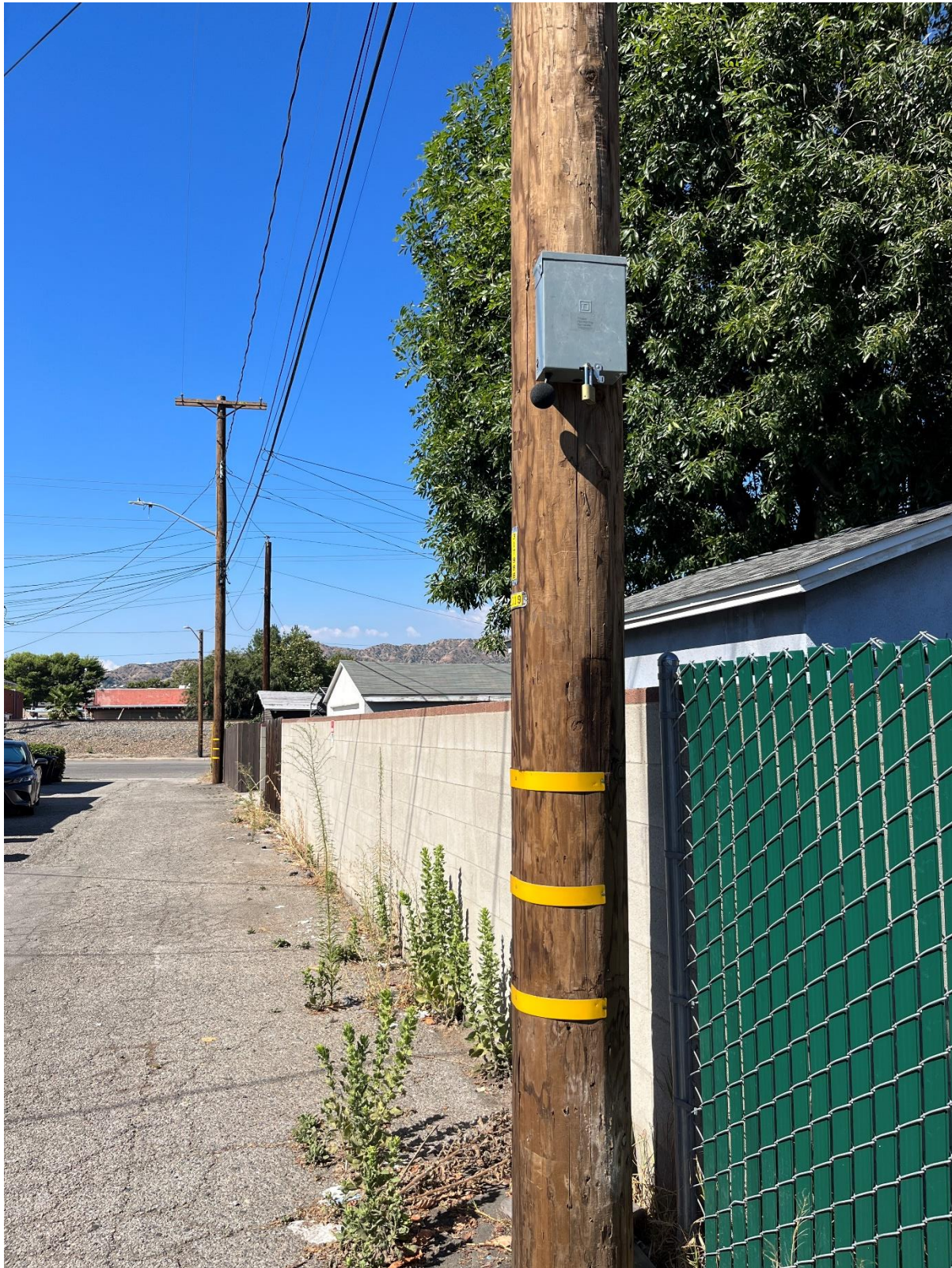
Figure 4 Sound meter installation at measurement location 3
